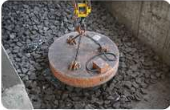
Scrap Charging In Induction Furnace
